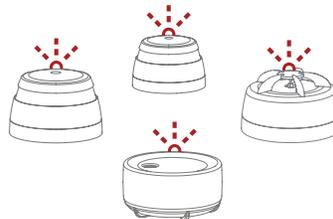
When the red LED light flashes on all alarms, they are connected and **MUST BE SWITCHED OUT OF 'LEARN MODE'** and installed.
