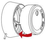
Turn the alarm until it clicks all the way in and can't be turned - then it is correct position.
