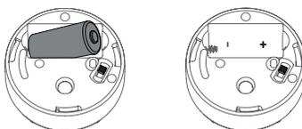
To replace the battery, detach the cover of the flood alarm by twisting counterclockwise.
