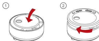
Remount the Test button / Lid. Close the flood alarm top cover by twisting clockwise.
