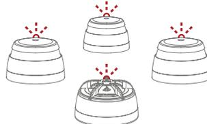
When the red LED light flashes on all alarms, they are connected and **MUST BE SWITCHED OUT OF 'LEARN MODE'** and installed.
