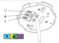
Install the cableholder and replace the cover.
