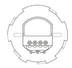
Screw the power supply on conduit box.
