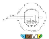
Connect the 3 wires to the power supply: Live feed (L1), neutral (N), Ground  $(\bot)$ .
