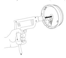
Install the power supply into the mounting base ring or use the conduit box as shown in option 1 & 2. **NOTE**: Alarm supply must be different from the lamp supply which can be switched ON and OFF.
