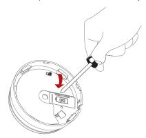
Replace the battery respecting the polarities.
