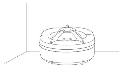
**NOTE:** If you place the flood alarm in places where a potential water leak / flood can rise higher than 2cm, there is a risk of your flood alarm being damaged. In these places we recommend wall mounting base with probe.
