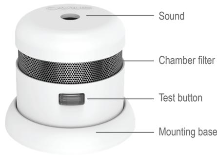
**Hush function:** In case of unintentional alarm condition or false alarms, press the side button. This will hush the alarm for 10 minutes, after which time it will automatically resume its normal alarm function.
