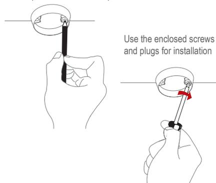
Use the enclosed screws and plugs for installation
