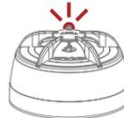
Please note that when the alarms are placed in 'Learn Mode' they can't be inserted into the mounting base. Do not take out the battery during 'Learn Mode' as this will interrupt the learn process.
