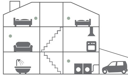
● Recommended CO alarm location
