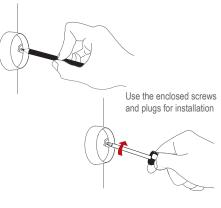
Attach the alarm by twisting clockwise.
