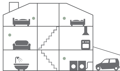
● Recommended CO alarm location
