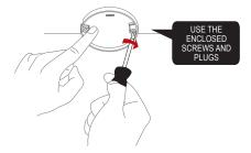
Once the mounting base is installed, attach the alarm by twisting clockwise until it clicks. If the switch is in 'Learn Mode', the smoke alarm will not be able to click into the mounting base.
